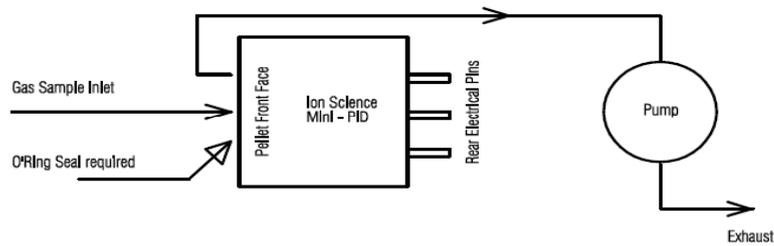
**Note:** Gauge pressures > +/-50 mbar, kPa will progressively dilute sample.
