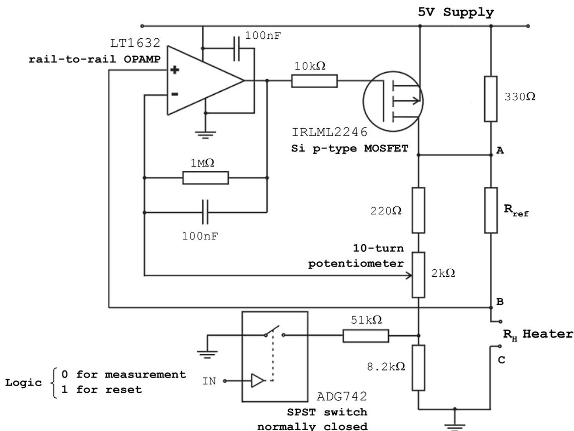
**Figure 2. Wheatstone Bridge Heater Circuit**
