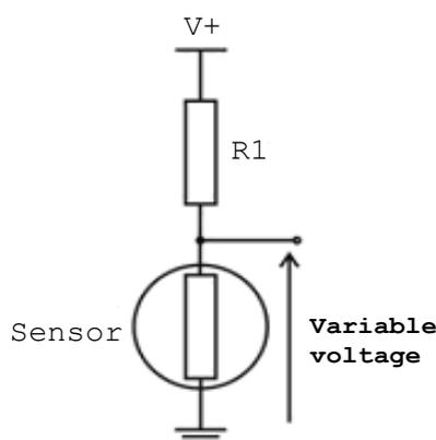
**Figure 3. Simple DC sensing circuit.**
