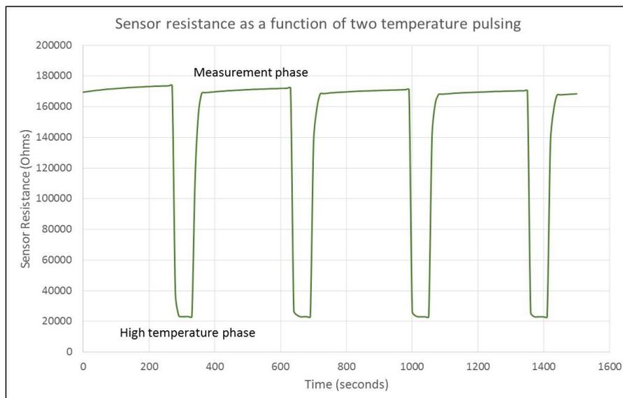
**Figure 1. Typical two-temperature pulsing profile for p-type metal oxide sensor**
