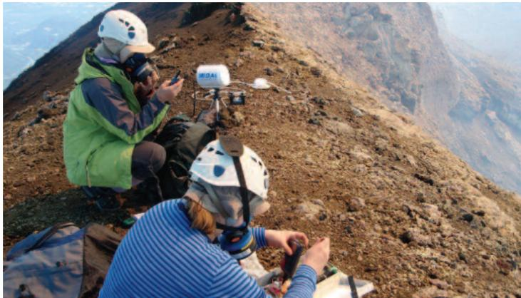
In developing our low-cost, low-power, high-durability instrument based on electrochemical sensors, we highlight the strong potential for electrochemical sensors to contribute to long-term volcano monitoring. The field-deployments demonstrated the capability of electrochemical sensors to endure the harsh, acidic environment of a volcano and to detect a range of gases in the plume-mixture, through newly developed
