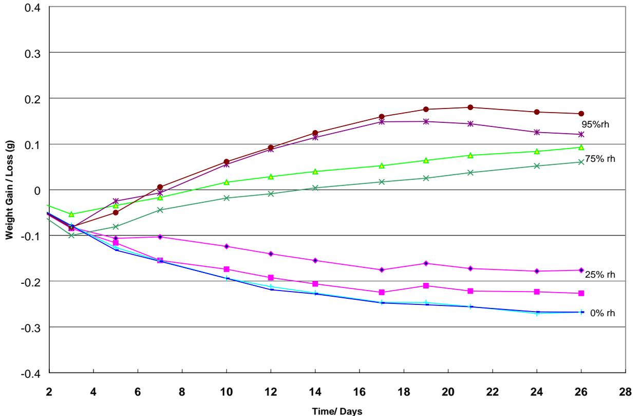
Figure 2. Sensor weight gain/ loss when subjected to humidity extremes.
