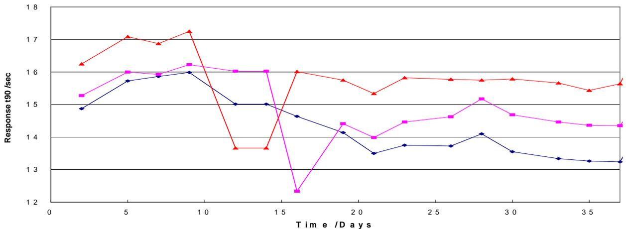
Figure 5. Response time ( $t_{90}$ ) stays constant for H<sub>2</sub>S sensors when losing water at 0% rh.
