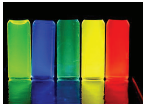
Figure 4. As CdSe/ZnS quantum dot size changes, so the luminescent wavelength also changes.
