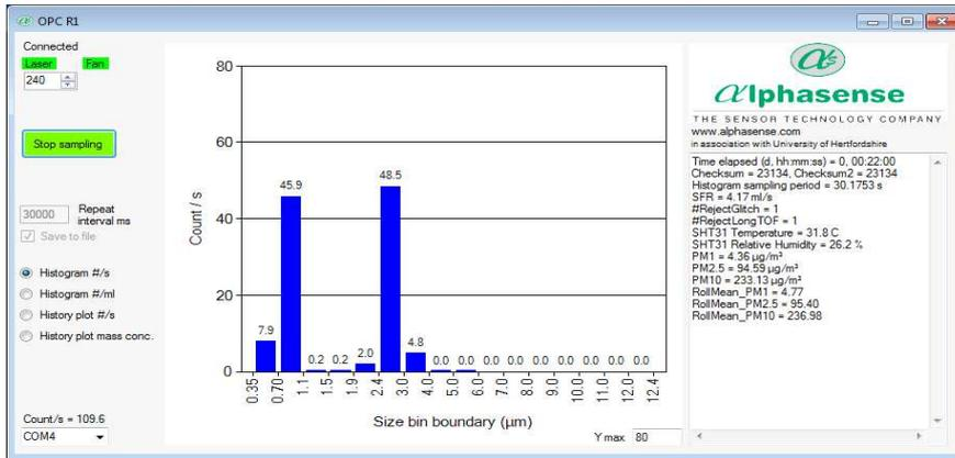
Figure 2 shows the OPC-R1 particle size distribution for the test aerosol.
