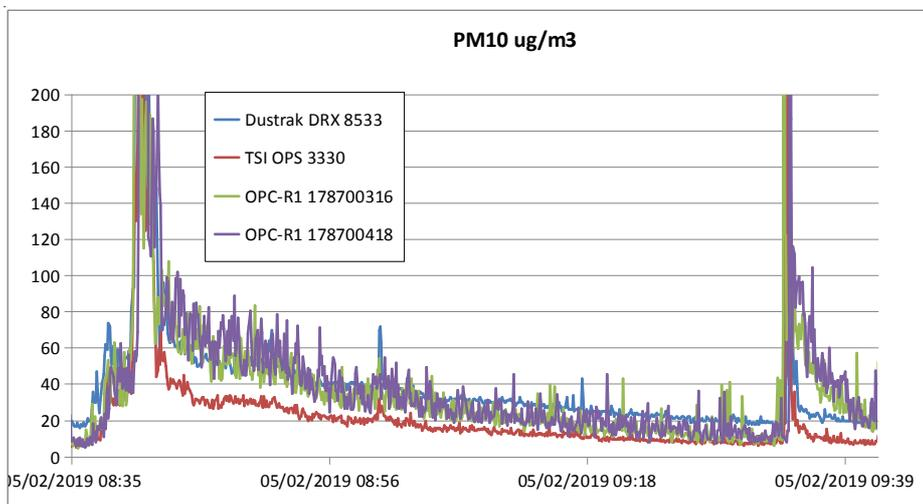
Figure 4 shows a comparison of PM10 monitoring by OPC-R1 sensor and TSI OPS 3330 and DustTrak instruments. All are set at 5s averaging and are sampling the ambient air of a work shop, the raw 3330 data has been used to calculate a PM figure.
