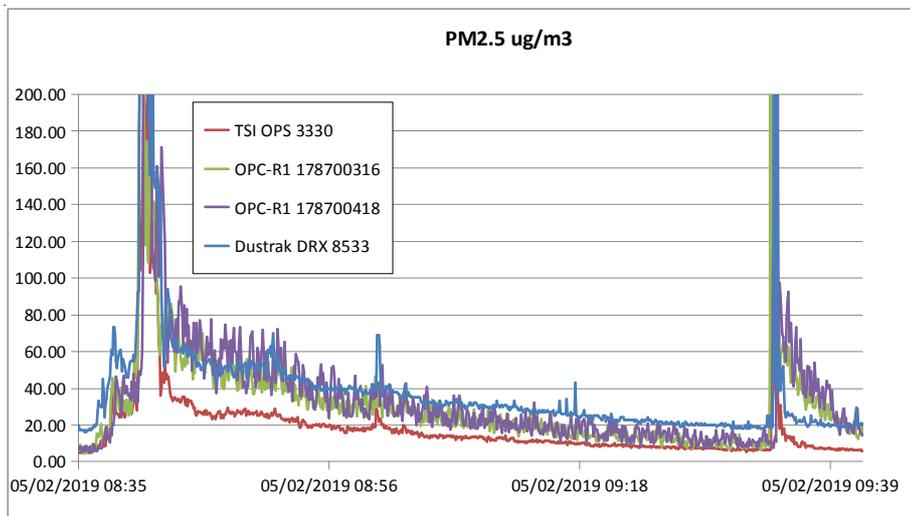
Figure 3 shows a comparison of PM2.5 monitoring by OPC-R1 sensor and TSI OPS 3330 and DustTrak instruments. All are set at 5s averaging and are sampling the ambient air of a work shop, the raw 3330 data has been used to calculate a PM figure.
