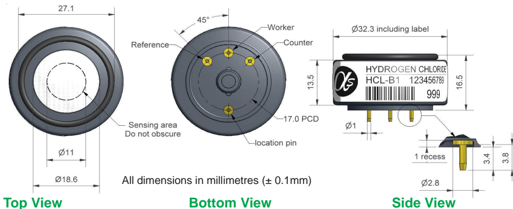
Figure 1 HCL-B1 Schematic Diagram
