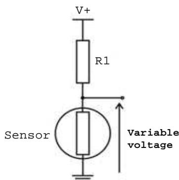
**Figure 3. Simple DC sensing circuit.**
