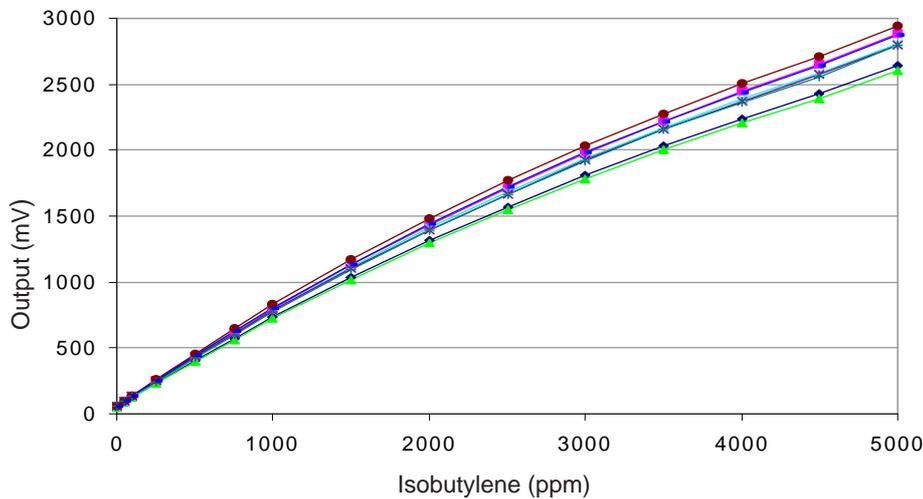
PID output is non-linear at higher concentrations but is repeatable and can be corrected in software.
