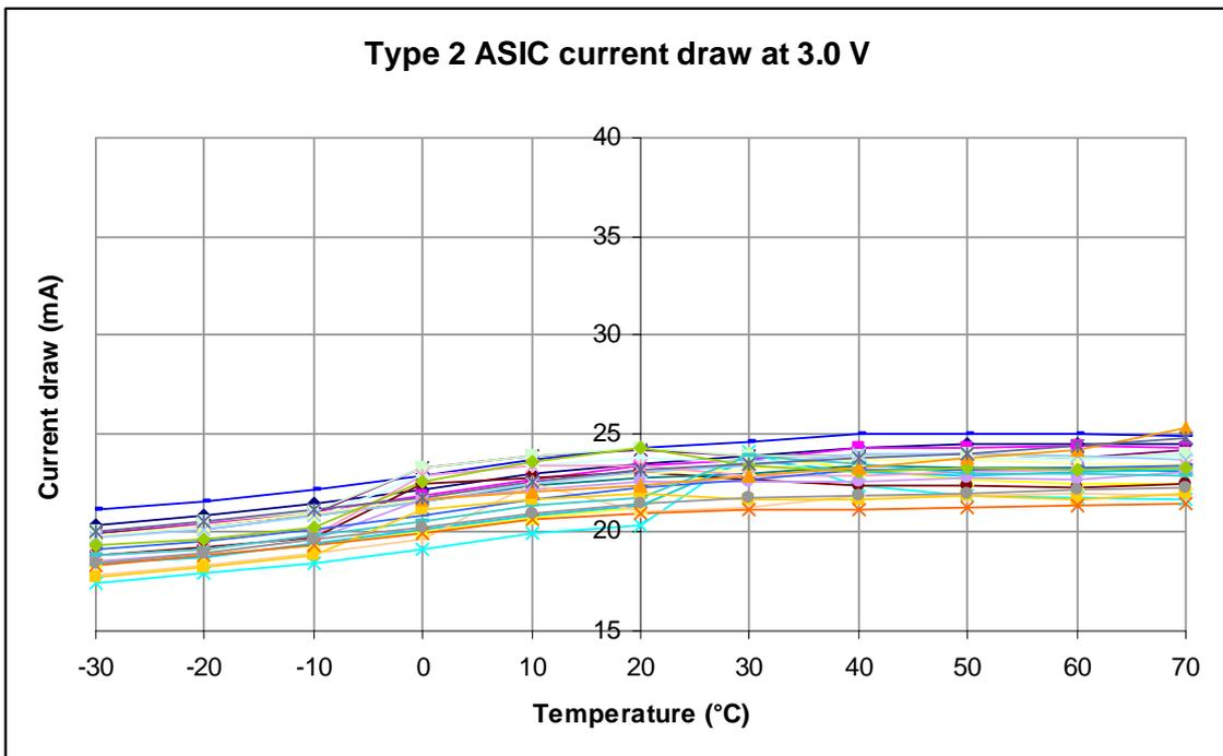
Figure 2. PIDs with the new ASIC show reproducible power consumption over a wide operating temperature enabling a greater degree of stability in your set-up.
