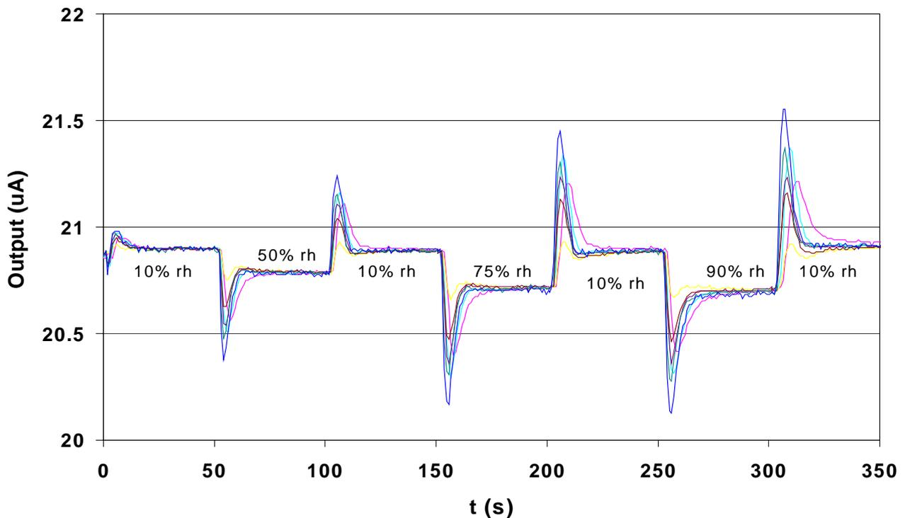
Figure 2. Transient humidity response of Alphasense O2-A1.
