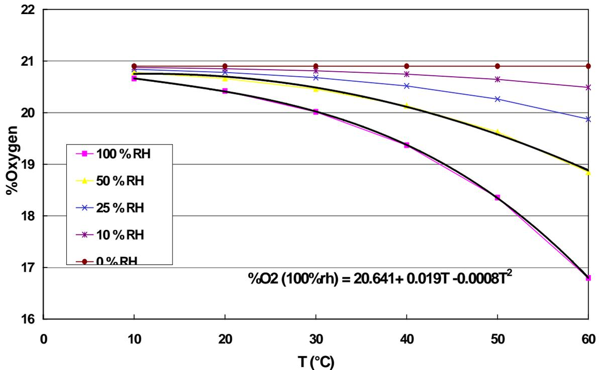
Figure 1 shows how oxygen concentration in air is diluted by humidity at different temperatures.
